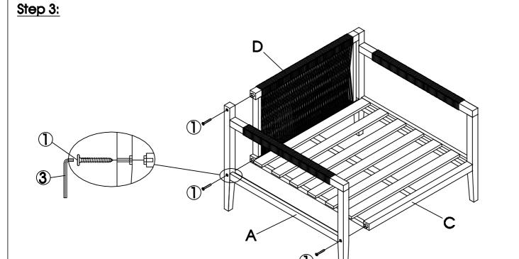
Fix the Left Leg Frame (A) to the Seat Panel (C) and Backrest (D) secure by using 03 screws (1) and Allen Wrench (3). Do not fully tighten the screws.
