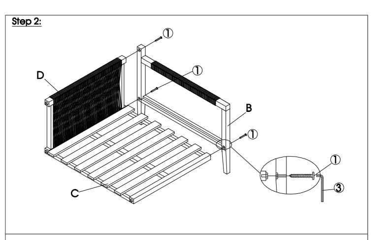
With the help of your adult partner, fix the Backrest (D), Seat Panel (C) with the Right Leg Frame (B) by using 03 screws (1) by Allen Wrench (3). Do not fully tighten the screws.
