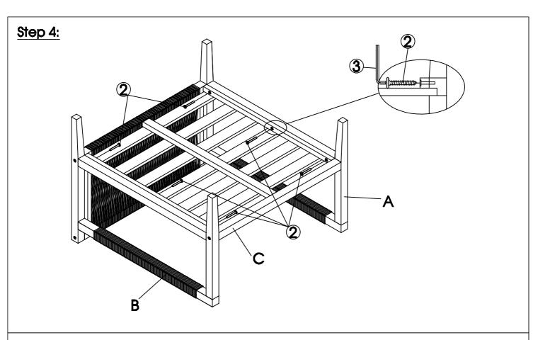
Fix the Seat Panel (C) with Leg Frame by using 06 Screws (2) by Allen Wrench (3). Do not fully tighten the screws.
