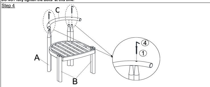
Turn the frame of step 3 right side up as shown in the picture above onto a clean, soft surface to avoid any scratches or damage to the product. With assistance from your adult partner(s):
