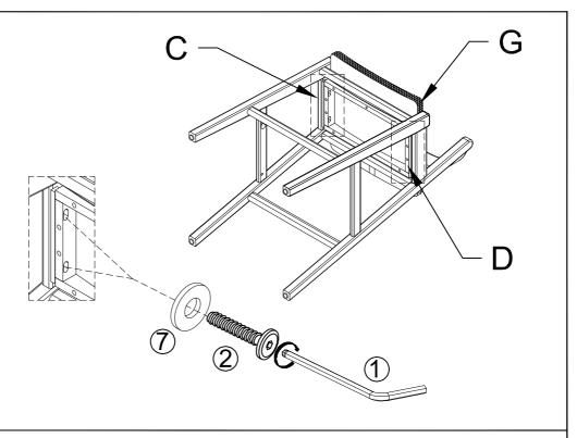
Use the Allen Wrench (1), Bolts (2), Flat washer (7) to affix the Seat Cushion with Top side bar (left) (C), Top side bar (right) (D). Tighten the Bolts.
