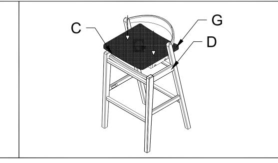
Place the Seat Cushion (G) into the Top side bar (left) (C), Top side bar (right) (D), so that the drilled holes of the Seat Cushion (G) coincide with Top side bar (left) (C), Top side bar (right) (D)
