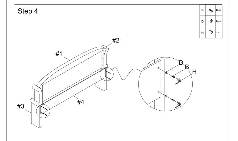
Assemble the Headboard bezel(4) to the back of the headboard
