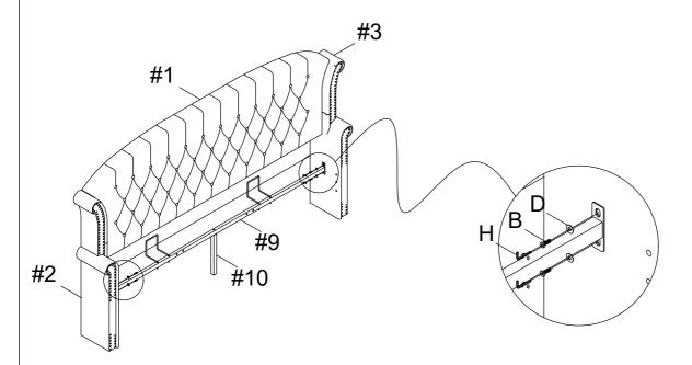
Assemble the rear crossbar (9) to headboard, contect to two bed ear
