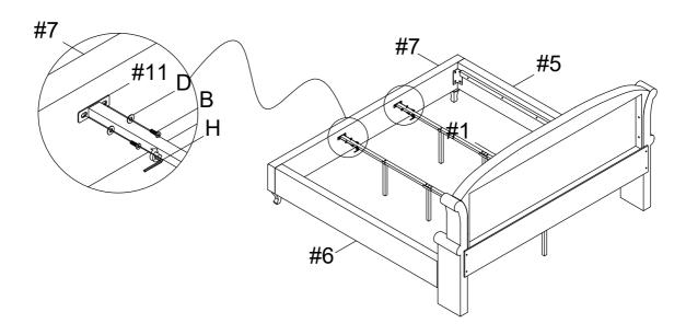
Assemble the 2 Vertical iron pipes (11) with footbaord(7)
