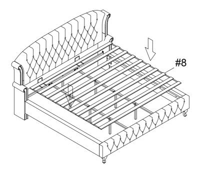
put the Rib strips (8) on the 2 Vertical iron pipes (11)
