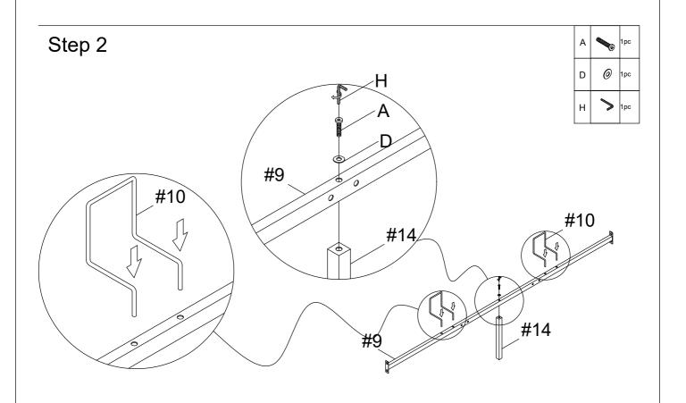
Assemble Rear gear bar(10) and ron feet (14) to Rear crossbar (9)
