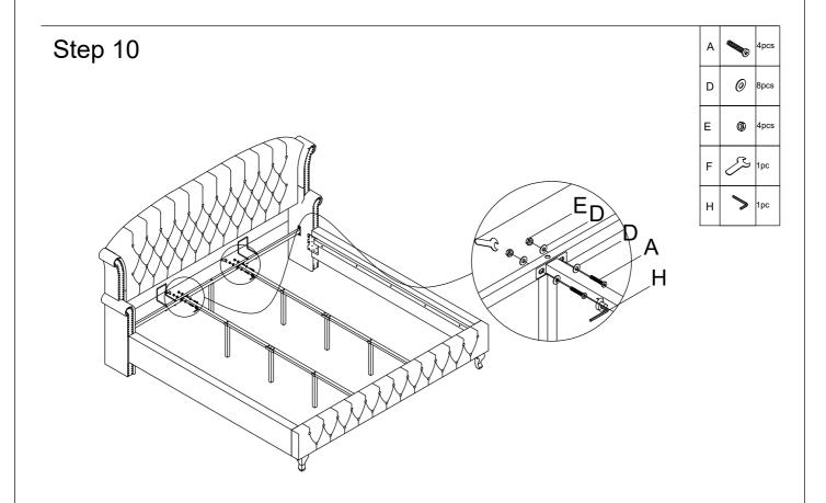
Assemble the 2 Vertical iron pipes (11) with rear crossbar(10)
