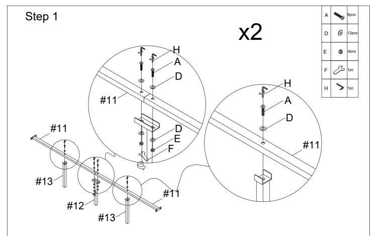
Assemble the Iron feet (12 &13 ) to Vertical iron pipes (11)
