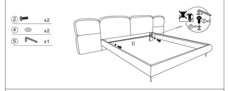
Attach the Cross Beam(H) to the Headboard Support Leg(DL & DR) using Bolts(2), Washer(4) and Allen Key(5).
