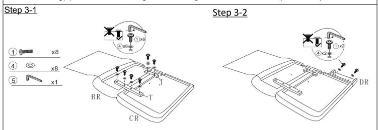
Connect the Upper Wing(BR) and Lower Wing(CR) with Wooden Batten(T&J) using Bolts(1), Washer(4) and Allen Key(5). Attach the Headboard Support Bar(DR) to the Lower Wing(CR) using Bolts(1), Washer(4) and Allen Key(5).
