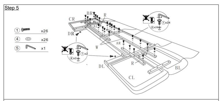
Place the Headboard(AL&AR) and two wings as shown above, align the holes of the Wooden Batten (W&R) to the parts, and tighten them with Bolts(1), washer(4)and Allen Key(5).
