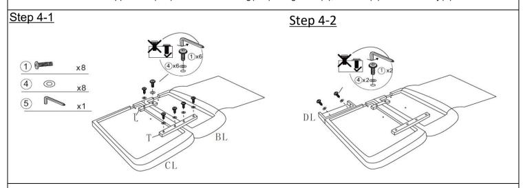
Connect the Upper Wing(BL) and Lower Wing(CL) with Wooden Batten(T&J) using Bolts(1), Washer(4) and Allen Key(5). Attach the Headboard Support Bar(DL) to the Lower Wing(CL) using Bolts(1), Washer(4) and Allen Key(5).
