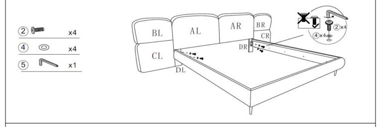
Attach the bed frame to the Headboard Support Leg(DL & DR) using Bolts(2), Washer(4) and Allen Key(5).
