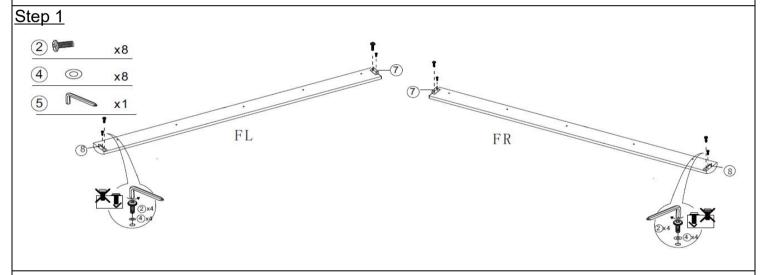
Attach Connector Plate(7) and Angle Bracket(8) to the Bedside Panel(FL) using Bolts(2) with Allen Key(5). Repeat the same step for another side.
