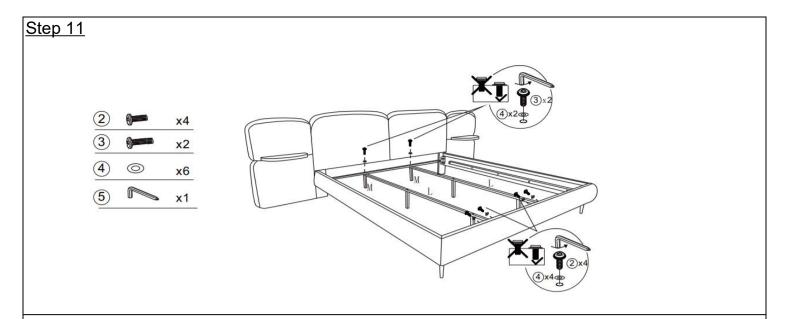
Connect the Support Rail to the cross beam and the footboard, fix it to the crossbar with Bolts(3), and fix it to the footboard with Bolts(2).
