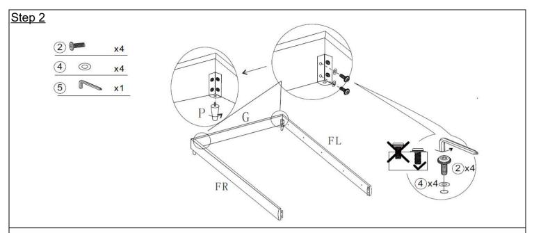
Attach the Footboard(G) to Bedside Panels(FL&FR) using Bolt(2) and Allen Key(5).
