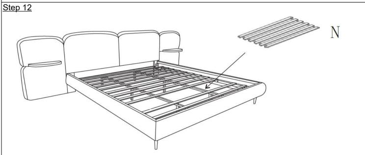
Unfold the slats and place on the bed frame.
