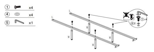
Attach the Support Leg(M) to the Support Rail(L) using Bolts(1), Washer(4) and Allen Key(5).
