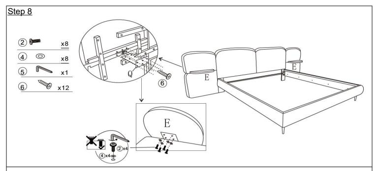
As shown in the picture above, insert the Metal Plate(Q) from the back to the front into the gap between the bed wings. Tighten the Metal Plate to the wooden batten using Screw(6) and Allen Key(5). Attach the Wing Panel(E) to the metal plate using Bolts(2), Washer(4) and Allen Key(5).
