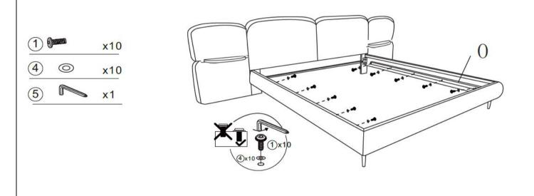
Attach the Slat Rail(O) to the bedside panel using Bolts(1), Washer(4) and Allen Key(5).
