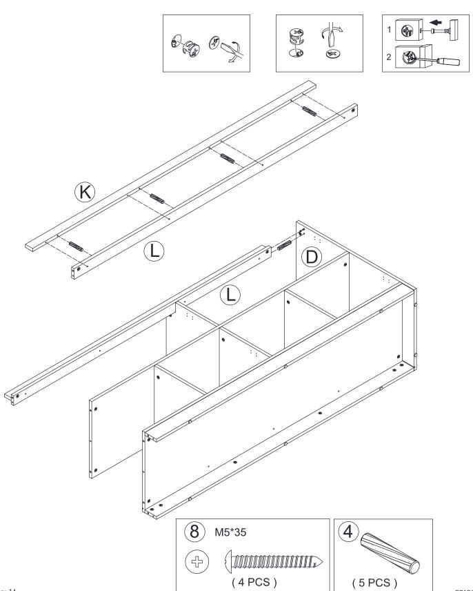
Attach the Left Side Panel (C) to the Bottom Panel (B), the Middle Panel (E), and the Middle Front Cross Panel (L) by using five pieces WOOD DOWEL (4) and fasten the HIDDEN CAM (2).
