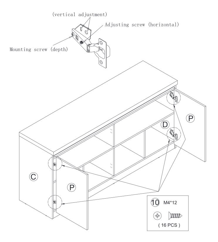
Fasten eight pieces of the FLAT HEAD SCREW (10) to fix the HINGE (6) to the Middle-Left Door Panel (Q) and Middle-Right Door Panels (P).
