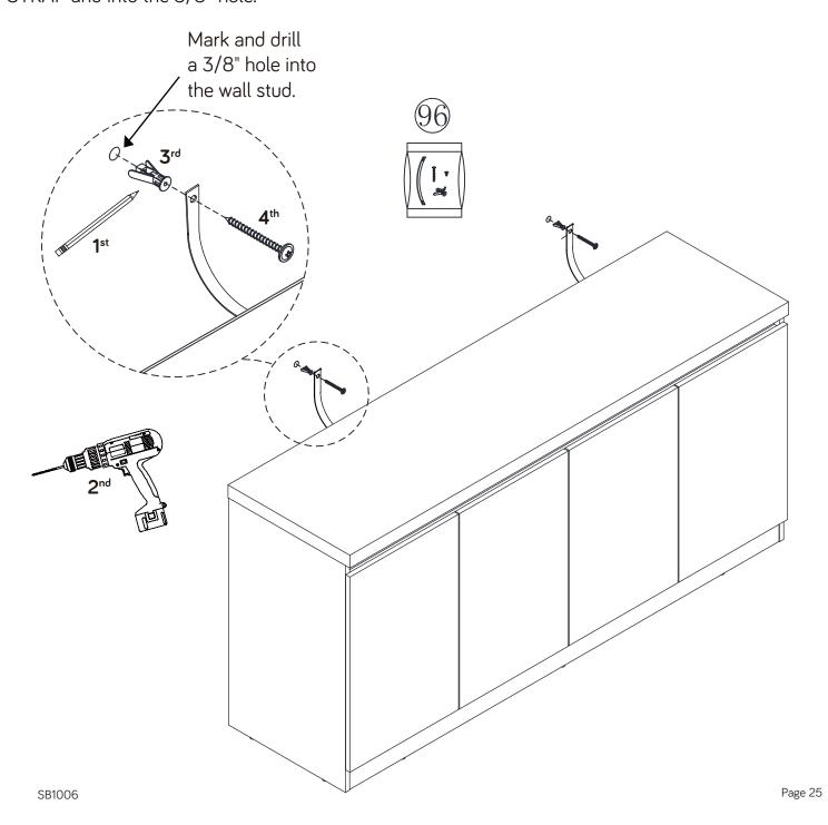
1st- With your pencil, strike a mark through the center of the hole in the SAFETY STRAP. 2nd- Drill a 1/8" hole on the mark.
