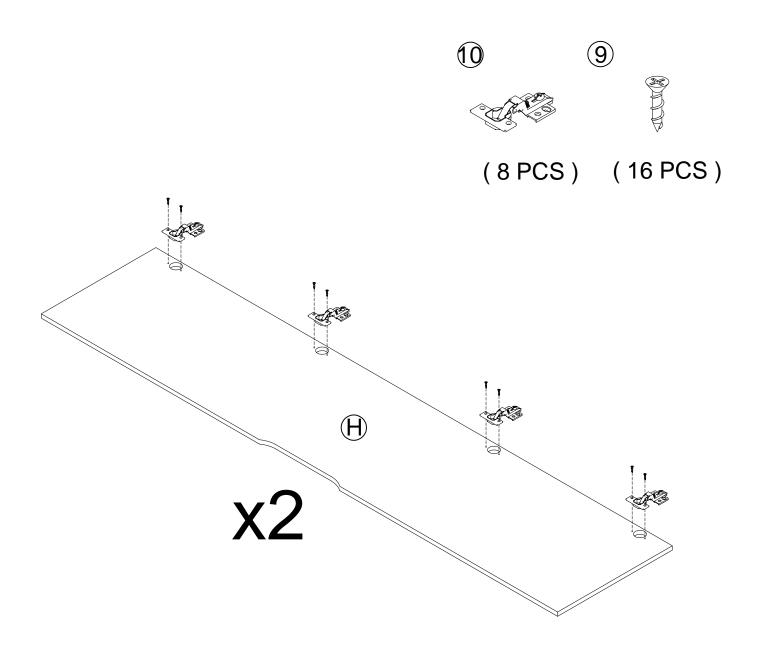
\* Attach the Two DOOR PANEL (H) to the stand with the SCREW (9) .
