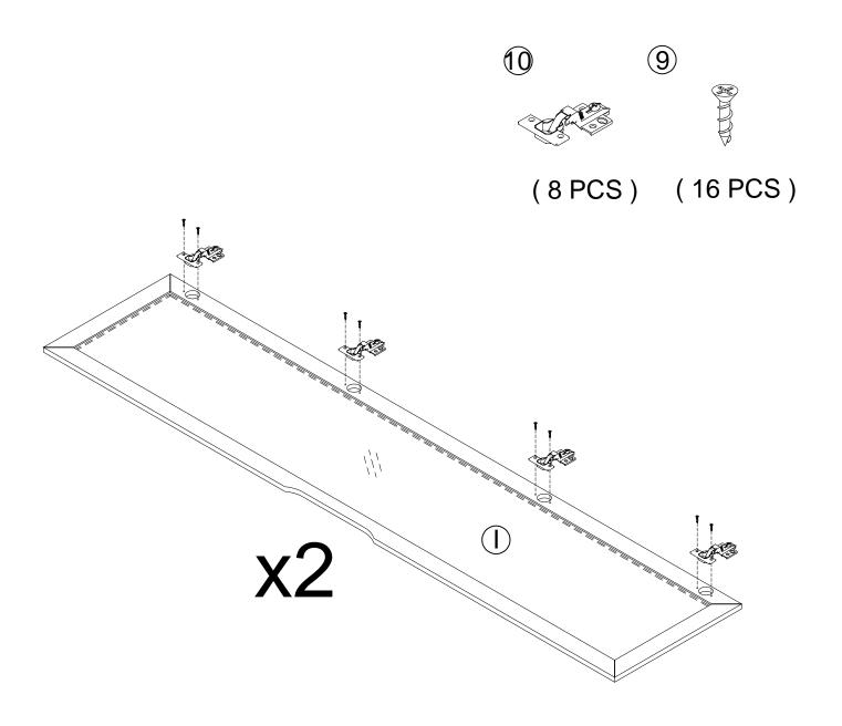
\* Attach the Two DOOR PANEL (I) to the stand with the SCREW (9) .
