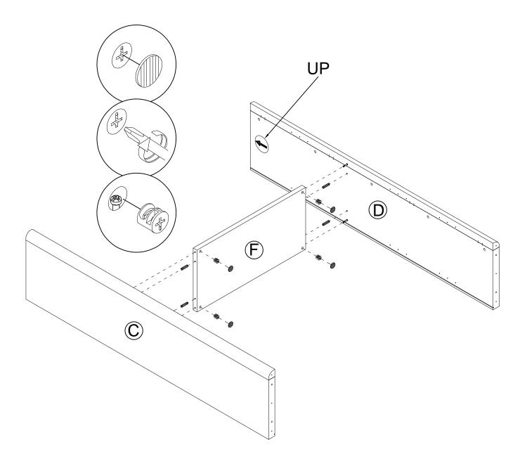
\* Attach the BOTTOM PANEL (B) to the LEFT PANEL (C) and RIGHT PANEL(D) by the Six Screw(8), Four WOOD DOWEL (4) and LOCK(7) .
