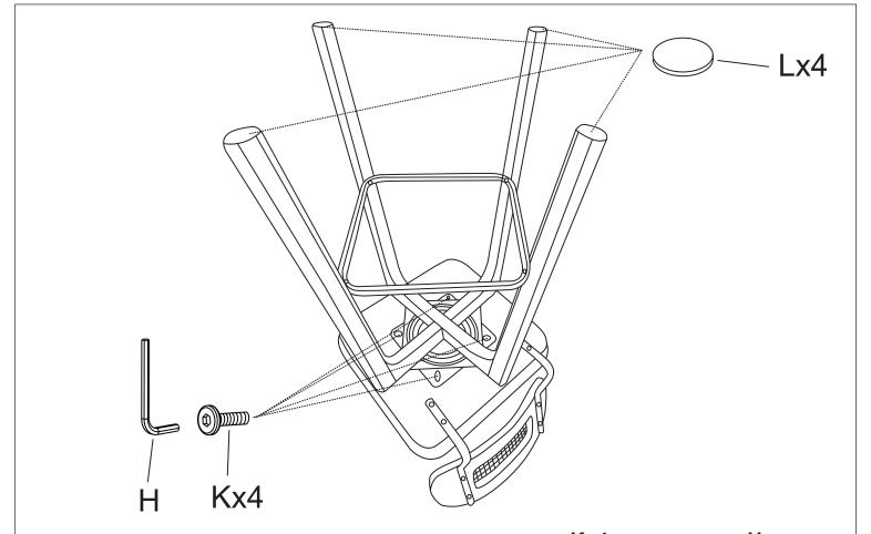
**Step 5**: Connect the Chair Leg and the Seat with Screws **Kx4** by Allen Wrench **H**. Paste the Foot Pad **Lx4** to the bottom.
