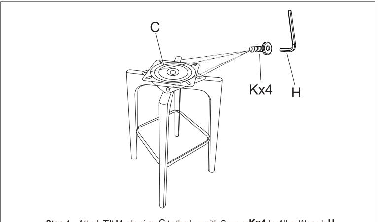
**Step 4**: Attach Tilt Mechanism C to the Leg with Screws **Kx4** by Allen Wrench **H**.
