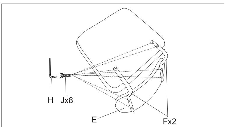
**Step 1**: Attach Back **E** to Seat **D** with Frames **Fx2** and Screws **Jx8** by Allen Wrench **H** as the picture. **Note:** Do not tighten completely until all screws are in place.
