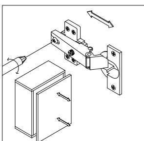
If the hinge holes are not aligned, you can try adjusting the front and rear hinges.
