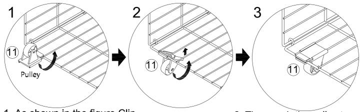
1. As shown in the figure Clip the pulley into position first
