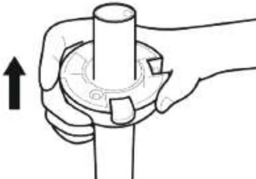
❸ Take off the hanging ball from the original downrod.
