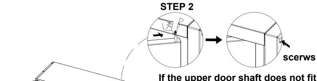
If the upper door shaft does not fit into the position shown in the illustration, you can send off the top screw on the same side and then install it (the screws are pointed out by arrows).
