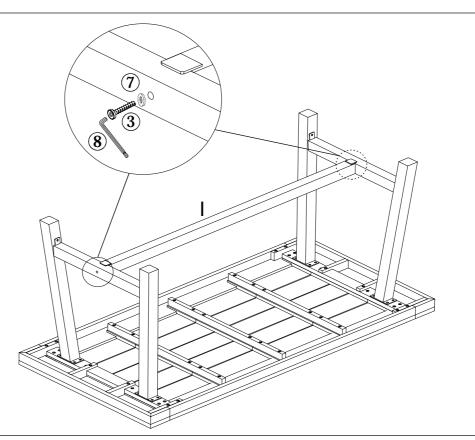
With the help of your adult partner, attach the Support Bar (I) to the Support Leg (H) by using 2 Bolts (3) and 2 Flat Washer (7) with Allen Wrench (8) as shown in the picture above.
