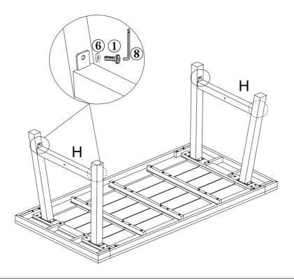
With the help of your adult partner, attach the Support Leg (H) to the middle of First Leg (F) and Second Leg (G) by using 2 Bolts (1), 2 Flat Washer (6) with Allen Wrench (8) as shown in the picture above.
