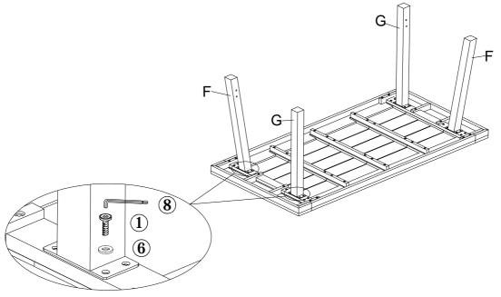
Attach the First Leg (F), Second Leg (G) to the Table Wings Panel (C) by using 4 Bolts (①), 4 Flat Washer (⑥) with Allen Wrench (⑧) as shown in the picture above.
