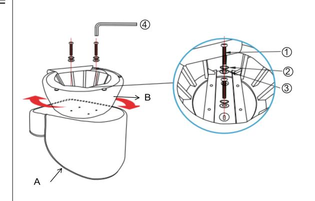
Rotate to align the remaining screw holes for installation. Secure with 2 Bolts (1), 2 Spring Washer Rings (2), 2 Flat Washer Rings (3) and Allen Wrench (4).
