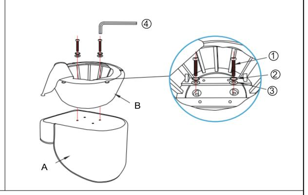
Rotate the base to align with the holes as the picture.
