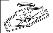
Hang the hole of the motor cover into the hook of mounting plate. FROM POWER SOURCE AC 110- 120 VOLT 60Hz 3.5AMPS.
