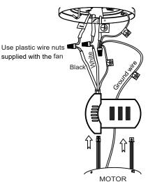
WARNING: To avoid possible electrical shock, be sure electricity is turned off at the main fuse box before wiring.
