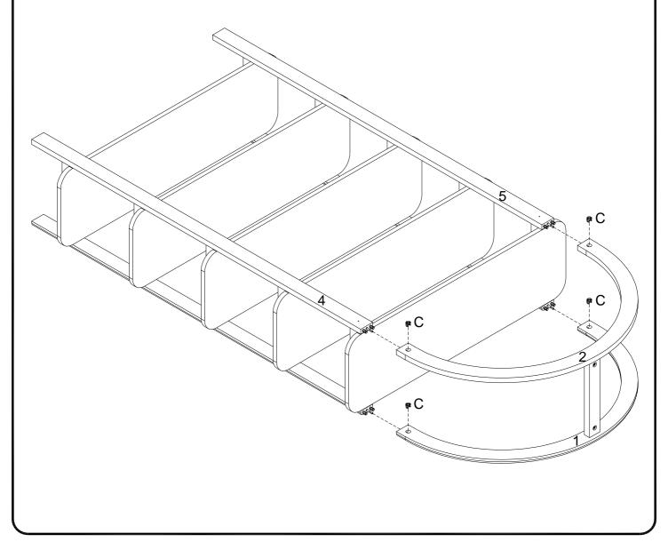
Use the provided stickers (D) to cover each cam lock (C) and ensure a clean finish.
