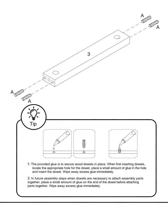
Next, insert wooden dowels (A) into each of the Support Bars (7).
