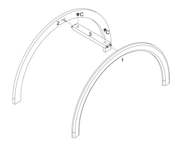
Now, attach the Top Arched Front Rails (1 and 2) to the top of each Side Frame (4 and 5). Insert cam locks (C) and tighten with a screwdriver.
