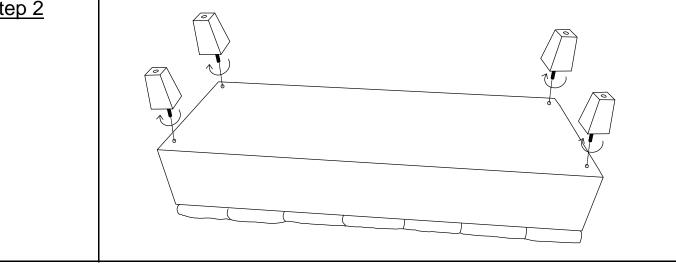
With assistance from your adult partner, place the Ottoman Body(B) face down as pictured on a clean surface. As shown in the picture, align the leg screw with the hole and tighten it in clockwise.
