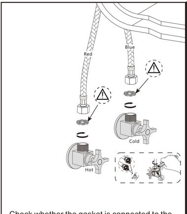
Check whether the gasket is connected to the water inlet pipe by securing it with a wrench
