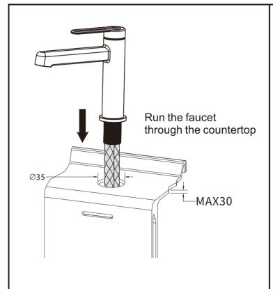
The recommended opening size of mesa is 35-40mm and the maximum thickness is 30mm
