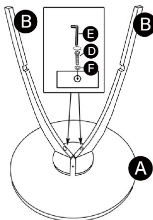
Flip the table top A upside down. Attach two legs B to the bottom of the table top A with screws and flat washers as shown.
