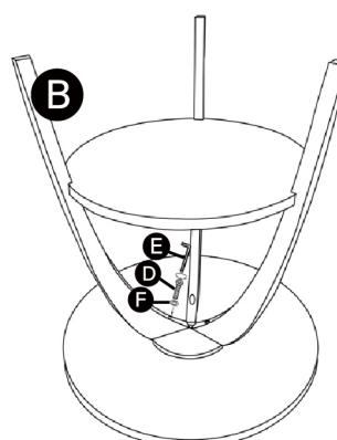
Attach the remaining leg B to the bottom of table top A with screws and flat washers as shown.
