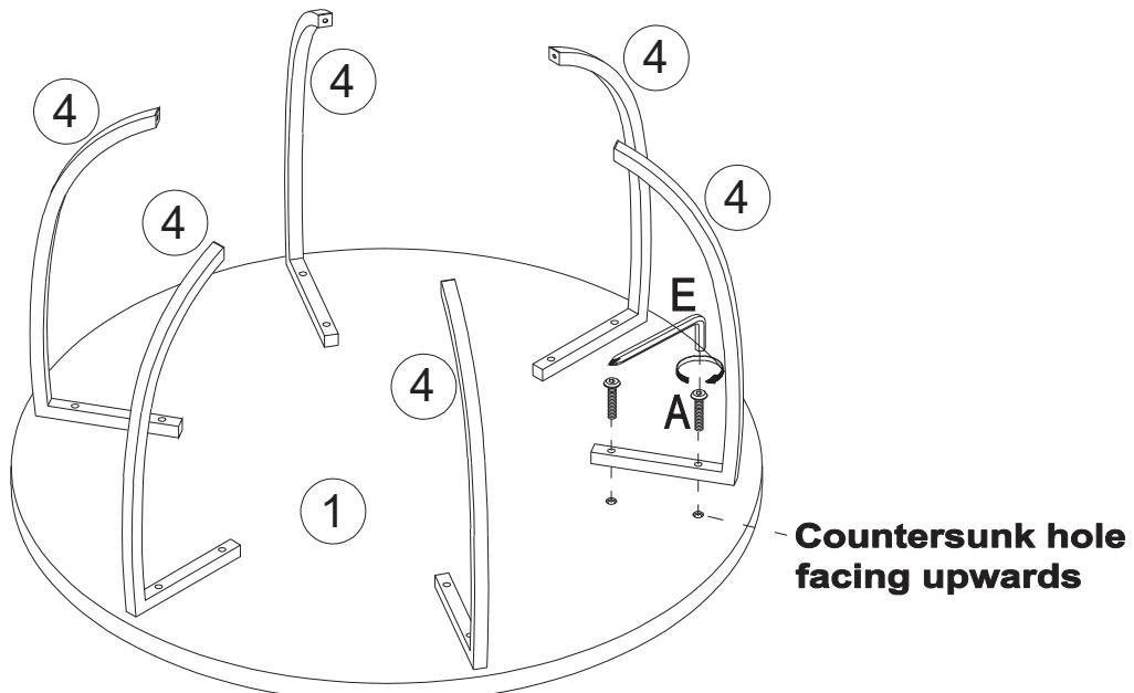
Tighten screws only after all parts have been property assembled.
