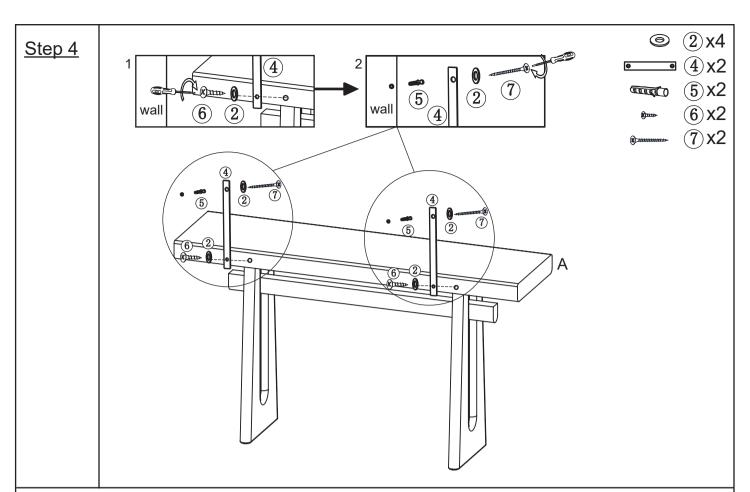
Attach the anti-tilt strap (4) to the top panel(A) with screw (6) and flat washer(2). Drill hole on the wallby using electric drill. Insert nut (5) into the hole. Attach the anti-tilt strap (4) to the wall with screw (7) and flat washer(2).
