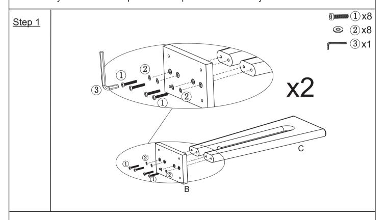
Attach the leg (C) to the panel(B), use bolt(1) and flat washer(2) align with board hole position, allen wrench (3) is used to assist rotation tightening.
