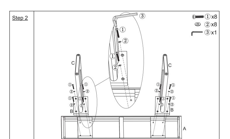
Attach the leg (B,C) to the top panel(A), use bolt(1) and flat washer(2) align with board hole position, allen wrench (3) is used to assist rotation tightening.
