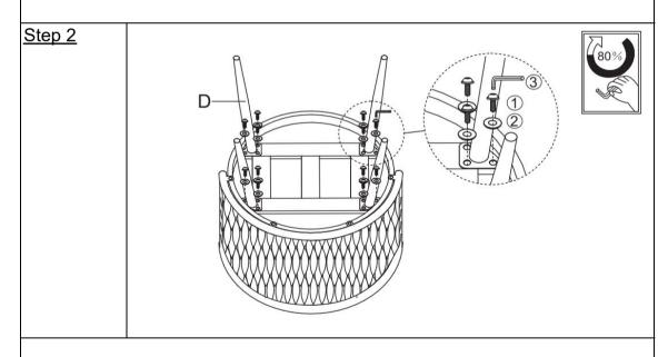
Attach the Leg (D) to assembled frame using the Washer (②) and Bolt (①) with Allen Wrench (③) as shown above.
