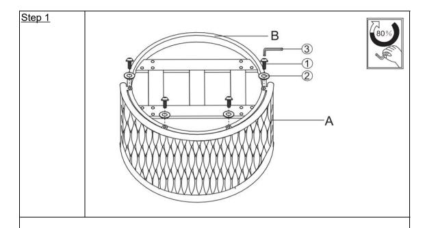
Attach the Connection (B) to Back (A) using the Washer (②) and Bolt (①) with Allen Wrench (③) as shown above.
