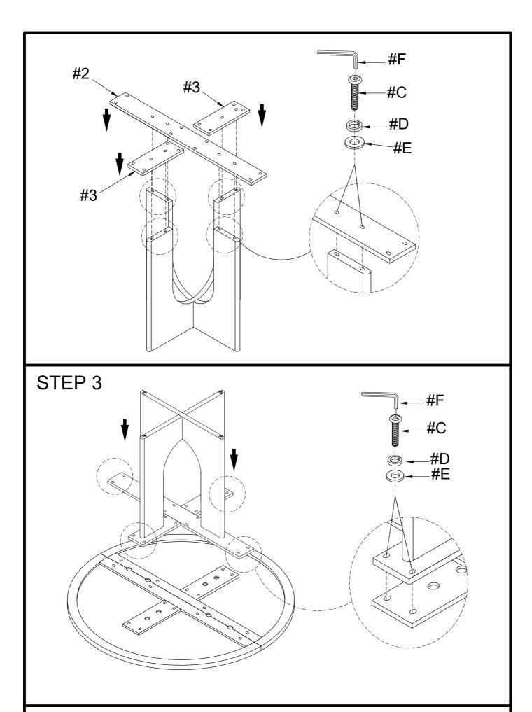
Do not tighten screws until completely asembled.
