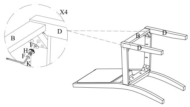
Take the Allen Wrench, and turn the bolts until the legs are secured. DO NOT TIGHTEN COMPLETELY.
