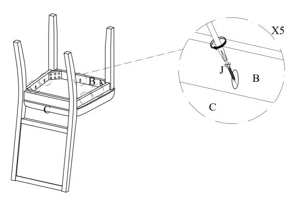
4 Stand the chair on an even surface and check for balance. If the chair wobbles slightly, apply downward pressure on the uneven leg and tighten the bolts to correct the imbalance. Once the chair is balanced, apply downward pressure evenly in the center of the chair and tighten all bolts, being careful not to over-tighten beyond the hole depth.
