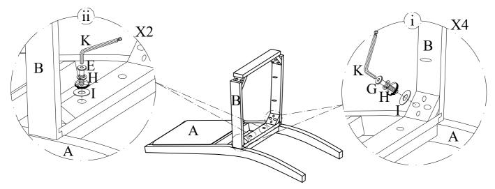
Take the Allen Wrench, and turn the bolts until the legs are secured. DO NOT TIGHTEN COMPLETELY.
