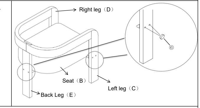
Cover the bolt holes with the Plastic cap(⑥).
