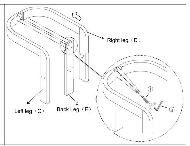
Attach the Back Leg(E) into the mounting positions of the Legs(C+D) using Bolts(1) with Allen Wrench(5).
