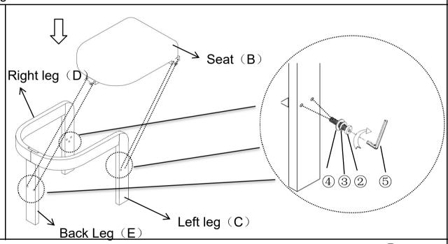
Attach the Legs(C+D+E) into the mounting positions of the Seat(B) using Bolts(2), Spring Washer(3) and Washer(4) with Allen Wrench(5). Do not fully tighten the Bolts.
