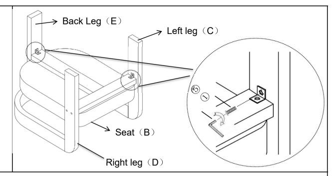
Attach the Legs(C+D+E) into the mounting positions of the angle iron using Bolts(1), with Allen Wrench(5).
