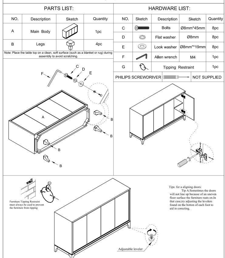
Note: Once all parts are aligned and properly in place, fully tighten all screws, and tighten gradually and evenly to avoid misalignment.
