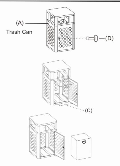
Use the key (D) open door to take out off inner liner (C)
