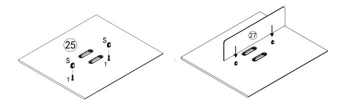
Install the screen into the screen clip.
