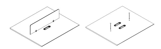
If the installation of a screen is not required, the hole cover can be installed over the hole on the countertop.
