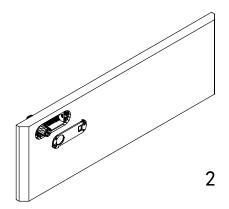
The screws of the lock need to be removed in advance.
