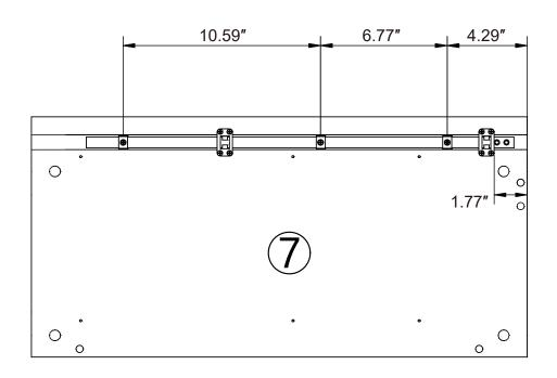
Recommended installation dimensions for the lock strip. Adjustments can be made based on actual conditions.
