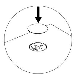
1. Peel off the protective film of the Ring-Mei Patch and align it with the hole (ensure the patch size matches the hole, with the patch slightly larger than the hole edges).
