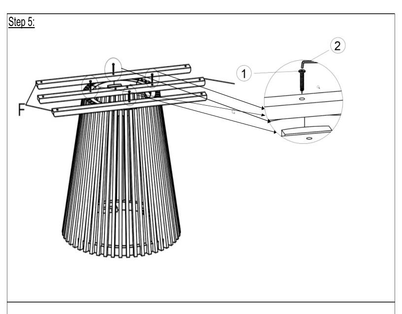
With the help of your adult partner, turn the assembled part in Step 4 right side up then place the Support Bars 1 and 2 (E, F) onto the above frame as shown above and secure by using Screw (1) and Allen Wrench (2).
