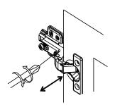
This is used to adjust the door panel in the up and down direction.
