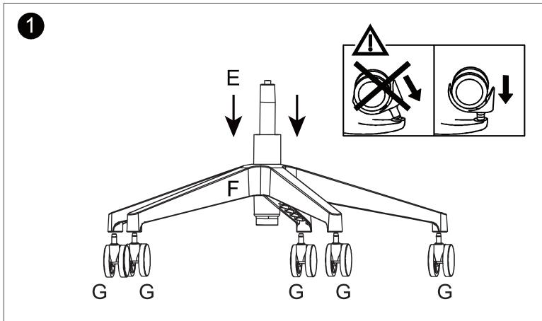
**Step 1**: Insert Casters Gx5 into the base with force. Insert the gas lift E into the center of the base.
