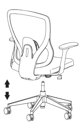
**Step 5** Align the assembled seat cushion with the assembled base, ensuring the holes on the seat chassis align with the top of the lifting gas spring. Then press down firmly to secure it in place.
