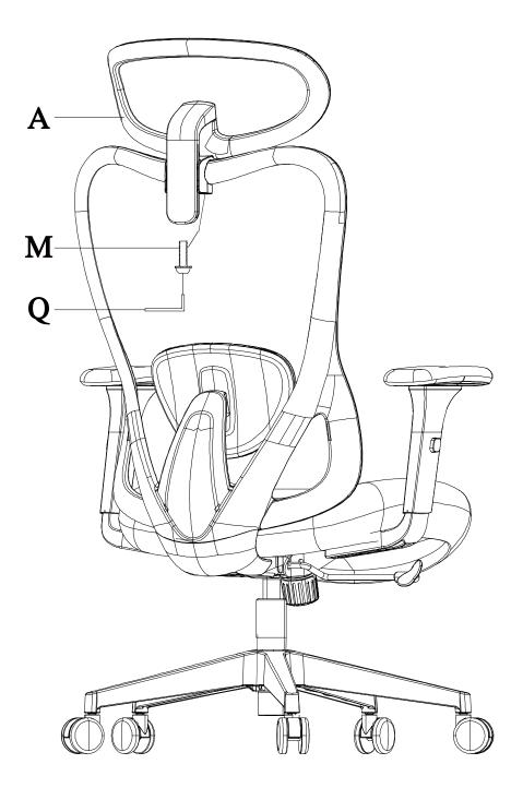
**Step 5** Attach the Headrest A to the Backrest with Screws Mx1.
