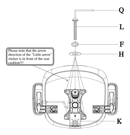
**Step 2** Attach the Tilt mechanism K to the Seat C with Screws Lx4, Screw gasket Fx4 and Hx4 as the picture.
