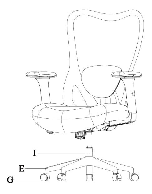
**Step 4** Insert Casters Gx5 into the Base E with force. Insert the Gas Lift I into the center of the base.
