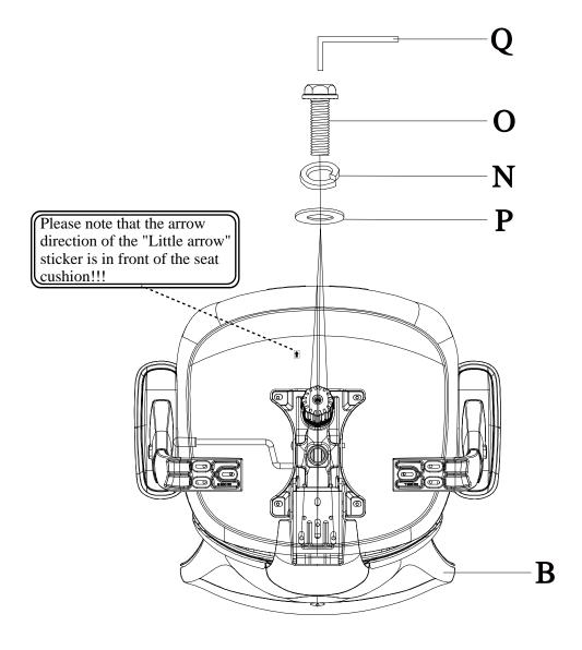
**Step 3** Attach the Back B to the Seat C with Screws Ox3, Screw gasket Nx3 and Px3 as the picture.
