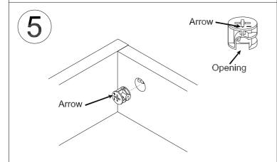
Insert the Cam Lock into the large hole. Make sure the arrow and the opening in the Cam Lock are facing the Cam Screw.
