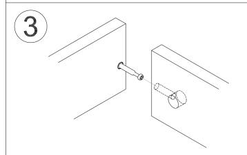
Connect the panels. Insert the Cam Screw into the small hole in the adjoining panel.
