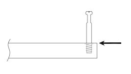
Screw the Cam Screw into the prethreaded hole. Tighten with a screwdriver until snug.
