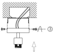
Screw the screw into the mounting board, and secure the light to the mounting board.
