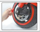
3. Install the front wheel: Connect the front wheel line with the body line; Penetrate into the body hole; Install the wheel covers on both sides.
