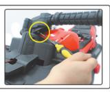
4. Installation of handlebars: Install handlebars; Insert screws and nuts; Tighten the fixing.
