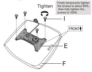
4 Assemble the installed base and seat.
