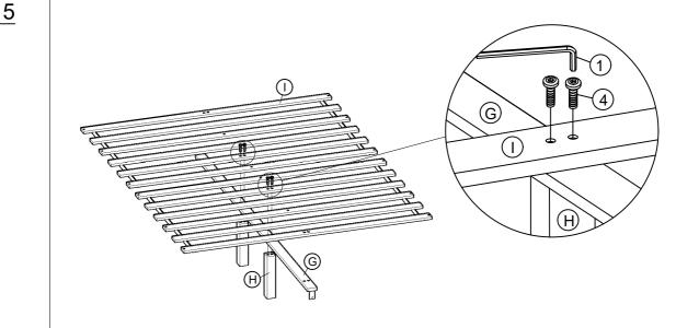
Align the Mounting Position on the Center Rail (G) to the Center Leg (H) and the Slat (I) Attach the Slat (I) and the Center Rail (G) to 2pcs middle Center Leg(H) by using Bolts (4) with M4 Allen Wrench(1)
