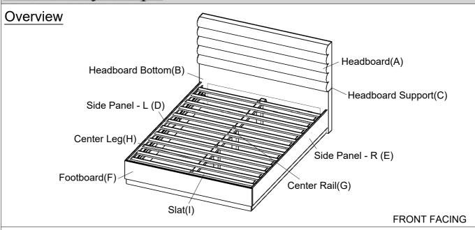
This Bed has multiple parts and may require up to 30 minutes to assemble. To give you an overview of the Bed parts, the above picture is provided to help you put the various parts into perspective. Please read through the instructions below to familiarise yourself with the parts and steps before assembly.
