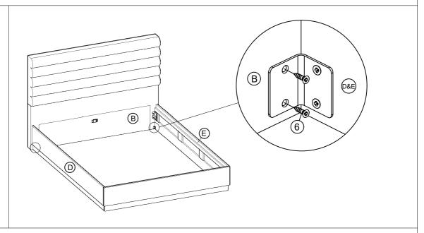
Screw up the iron panel on Side Panel L&R (D and E) to the bottom of headboard Bottom(B) using Screws (⑥) and Screwdriver (Not Provided).
