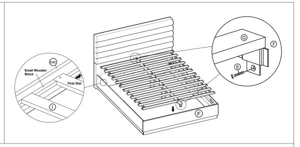
With the help from you partner, place the assembled Slats in the middle of the bed frame. Attention: When placing the Slats (I), please place the top 2pcs slats embed on the small wooden block in two ends of Side Panel L&R (D and E) as above picture shown, it will has the best performance of the slats.
