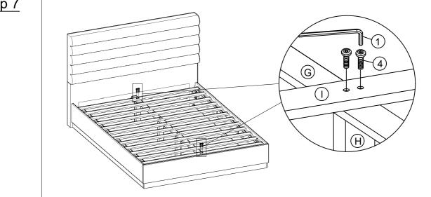
Attach the balance 2pcs Center Leg (H) to Assembled Slat (I) and the Center Rail (G) and by using Bolts (4), with M4 Allen Wrench(1).
