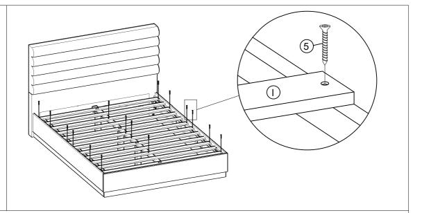
Attach all slats (I) to the rail on Side Panel L&R (D and E) by using Screws (⑤) and Screwdriver (Not Provided).
