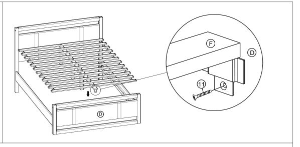
With the help from you partner, place the assembled Slats in the middle of the bed frame. Attach the Center Rail (F) to the Footboard (D) by using Screws ( $\mathfrak{I}$ ) and Screwdriver (Not Provided).
