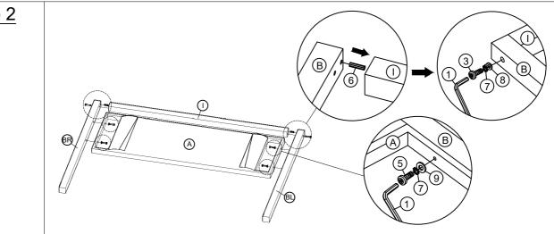
Place the Headboard (A) with its inner side face skywards onto a clean, soft surface to avoid any scratches or damages to the product.
