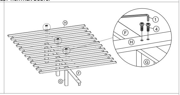
Align the Mounting Position on the Center Rail (F) to the Center Leg(G) and the Slat (H). Attach the Slat (H) and the Center Rail (F) to the Center Leg(G) and by using Bolts (4) with M4 Allen Wrench(1).
