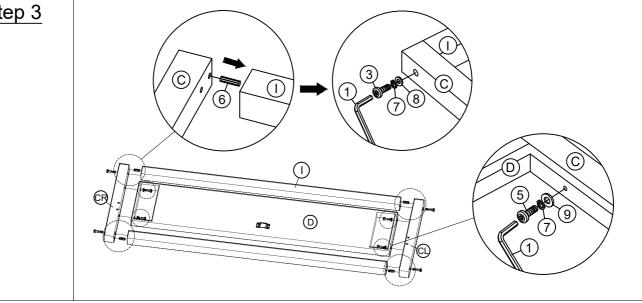
Place the Footboard (D) with its inner side face skywards onto a clean, soft surface to avoid any scratches or damages to the product.
