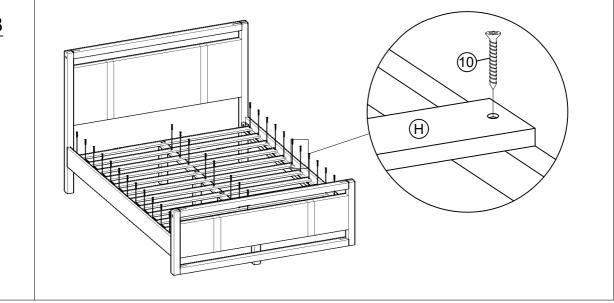
Attach all slats (H) to the rail on Side Rail (E) by using Screws (⑩) and Screwdriver (Not Provided).
