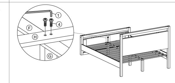
Attach balanced Center Leg(G) to Assembled Slat (H) and the Center Rail (F) and by using Bolts (4), with M4 Allen Wrench (1).
