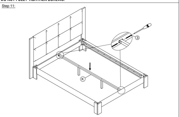
Attach Center rails support slats (K) with Metal link by using Screw and Screwdriver (Not Provided). DO NOT FULLY TIGHTHEN SCREWS. Page 9/11
