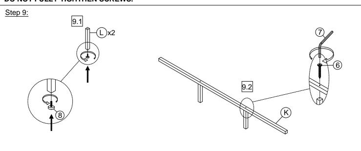
9.1: Attach Leveler® with Center support Leg (L) as shown above.
