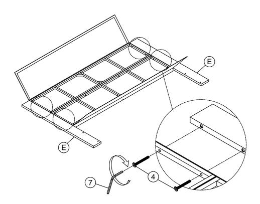
Attach Legs headboard (E) to the Headboard (A) by using Bolt(4)with Allen Wrench(7)as shown above. **DO NOT FULLY TIGHTHEN BOLTS.**
