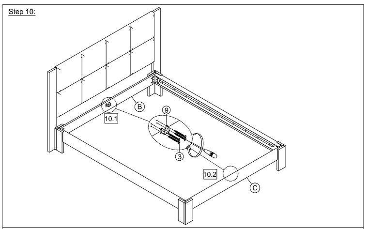
10.1: Attach Metal link with Crossbar-headboard (B) by using Screw and Screwdriver (Not Provided). 10.2: Attach Metal link with Bed rail (C) by using Screw and Screwdriver (Not Provided). **DO NOT FULLY TIGHTHEN SCREWS.**
