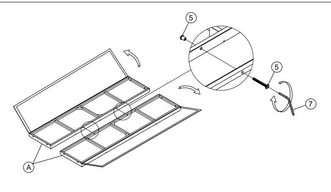
Open the pocket on back of headboard (A),attach 2pcs headboard (A) together by using Bolt with Allen Wrench as shown above
