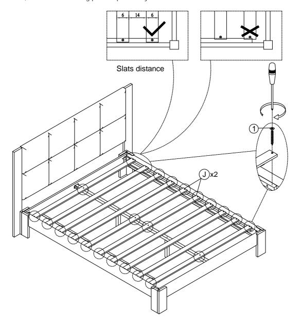
Attach Slats (J) to the Side rails (D) and Center rails support slats (K) by using Screws 1 and Screwdriver (Not Provided).
