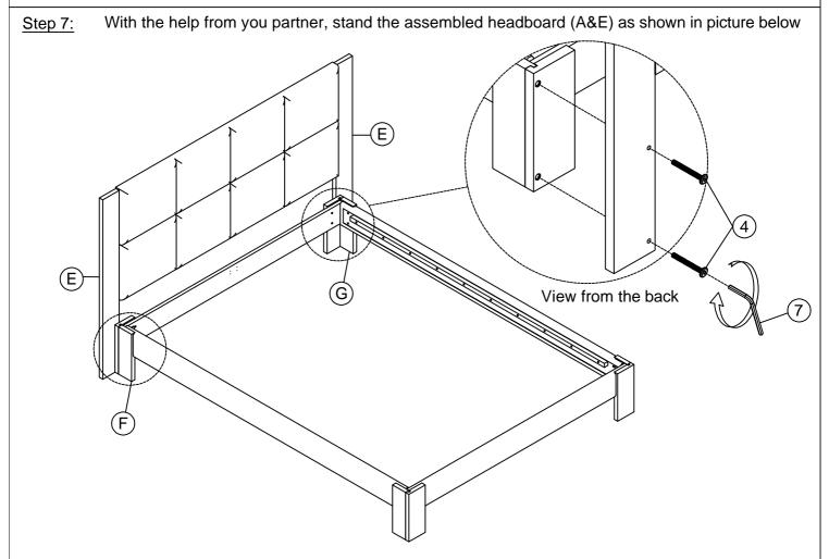
With the help from you partner, stand the assembled headboard (A&E) as shown in picture above Attach Legs headboard (E) to the Leg-left support headboard (F) and Leg-right support headboard (G) by using Bolt 4 with Allen Wrench 7 as shown above.
