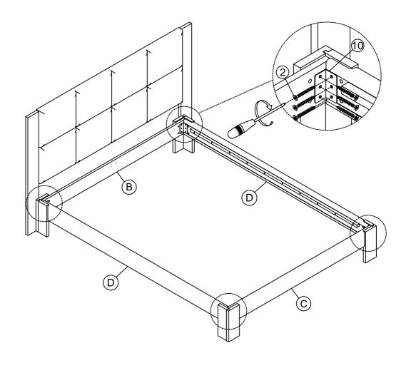
Attach Metal link 10 to the Crossbar-headboard (B), Bed rail (C), Side rail (D) by using Screws 2 and Screwdriver (Not Provided).
