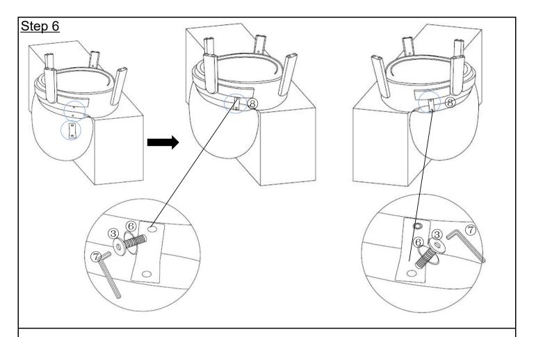
Take out L-shaped iron(8),asign it to the holes of the backrest as shown. Then use bolt(3) and Flat Washer(6) with Allen Wrench(7) to tighten it.
