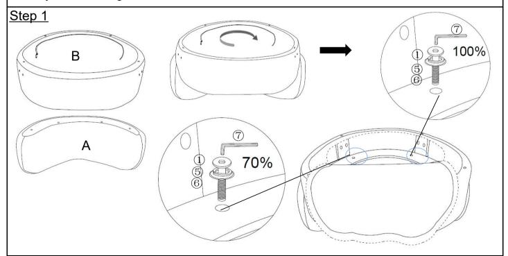
Take out Backrest(A) and Seat(B), attach Seat(B) to the Backrest(A) as shown.
