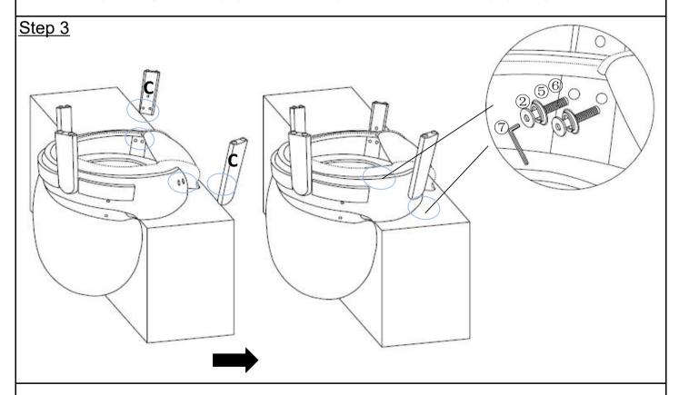
Take out Front Foot(C), align the holes to the front of the seat frame.
