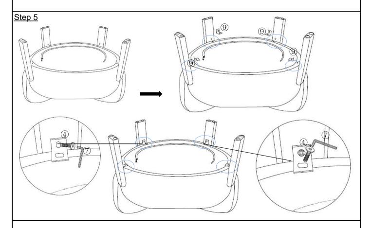
Take out L-shaped iron( $\mathfrak{P}$ ), asign it to the holes of the legs as shown. Then use bolt( $\mathfrak{P}$ ) with Allen Wrench( $\mathfrak{P}$ ) to tighten it.
