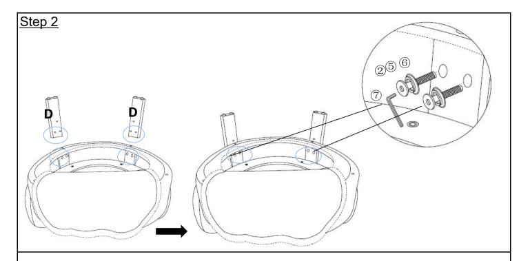
Take out Back Foot (D), align the holes to the back of the seat frame. Use Bolt (②), Spring Washer(⑤), Flat Washer(⑥) with Allen Wrench(⑦) to tighten it.
