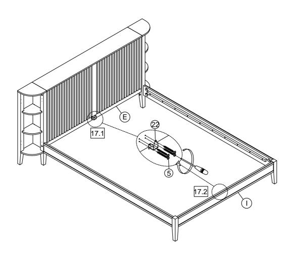
17.1: Attach Metal link 2 to the Bottom front crossbar-headboard (E) by using Screws 5 and Screwdriver (Not Provided).
