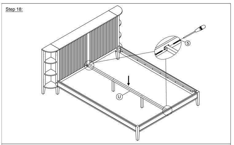
Attach Center rails support slats (U) with Metal link 2 by using Screws and Screwdriver (Not Provided). **DO NOT FULLY TIGHTHEN SCREWS.**
