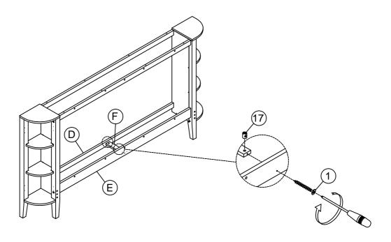
Attach Crossbar support headboard (F) to the Bottom back crossbar-headboard (D) and Bottom front crossbar-headboard (E) by using Screws①, Plastic nut ⑦ and Screwdriver (Not Provided).
