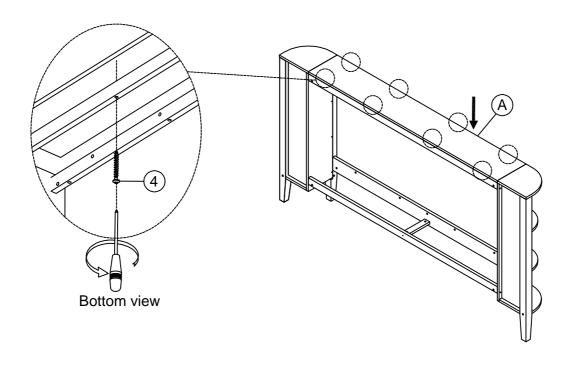
Attach Top headboard panel (A) to the Top back crossbar-headboard (B), Top front crossbar-headboard (C) by using Screws (4) and Screwdriver (Not Provided).
