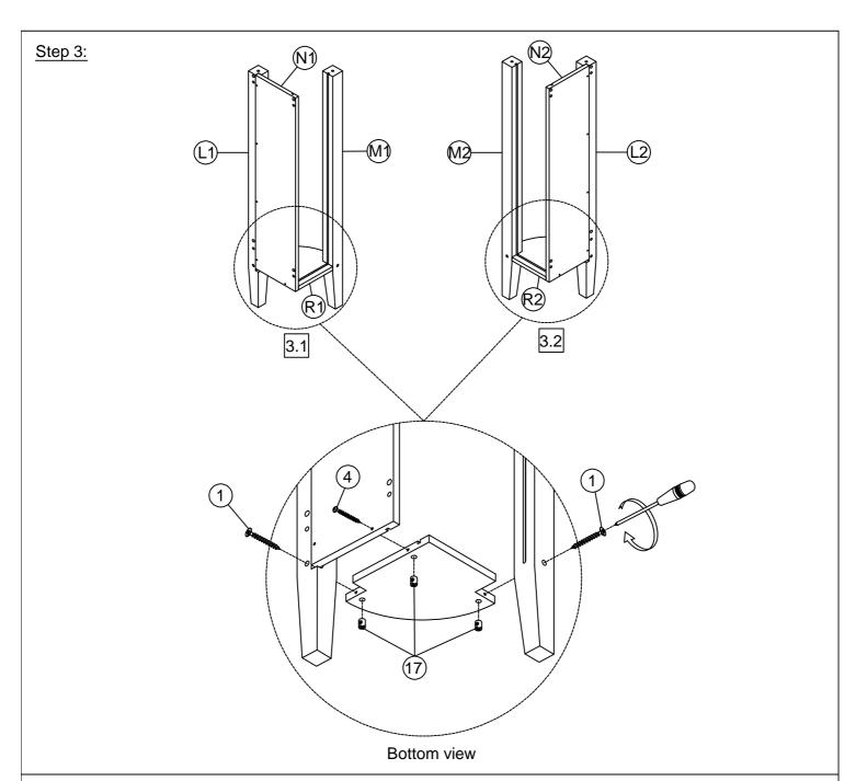
3.1: Attach Bottom left shelf panel (R1) to the Leg-left headboard (L1), Leg-left support headboard (M1) and Side left headboard panel (N1) by using Screws①, Screws②, Plastic nut① and Screwdriver (Not Provided).
