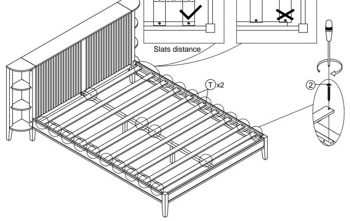
Attach Slats (T) to the Side rails (J) and Center rails support slats (U) by using Screws2and Screwdriver (Not Provided).
