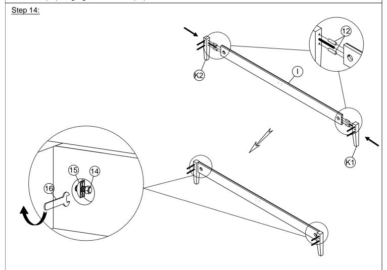
Attach Bed rail (I) to the Leg-left footboard (K1) and Leg-right footboard (K2) by using Wooden dowel ②, Hex nut (4), Half moon washer (5) with Open wrench (6) as shown above.
