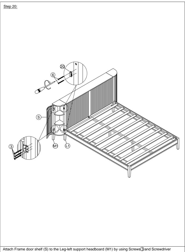
Attach Frame door shelf (S) to the Leg-left support headboard (M1) by using Screws(3) and Screwdriver (Not Provided).
