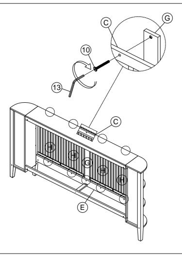
Attach Frame headboard (G), Frame headboard (H) to the Top front crossbar-headboard (C), Bottom front crossbar-headboard (E) by using Bolt (1) with Allen Wrench (13) as shown above.
