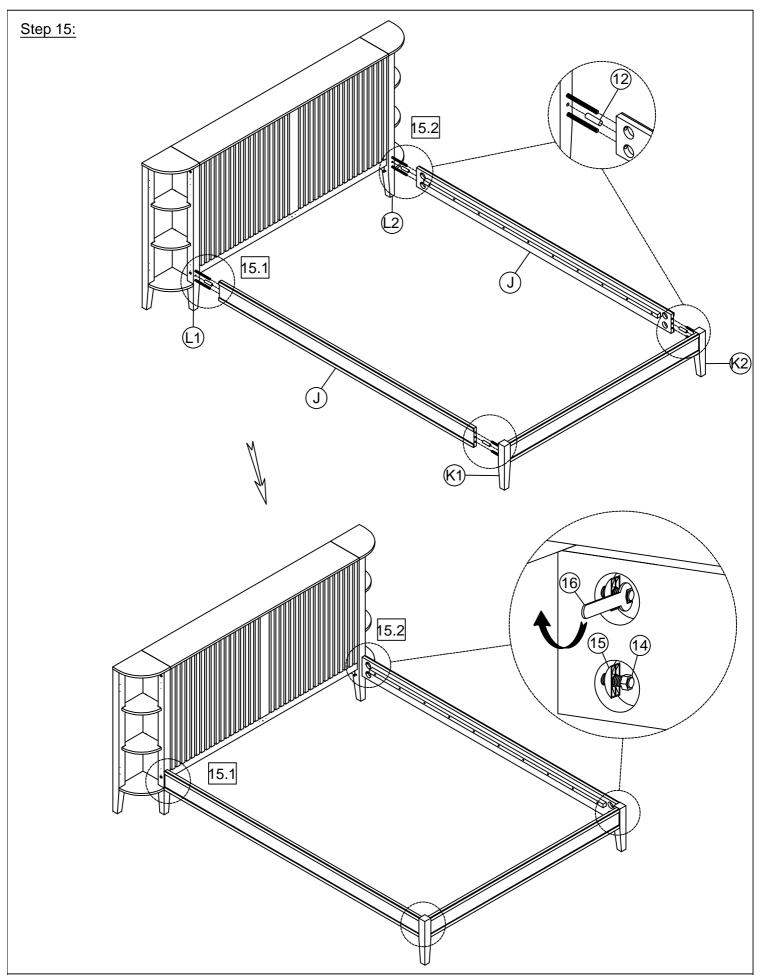
15.1: Attach Side rail (J) to the Leg-left footboard (K1) and Leg-left headboard (L1) by using Wooden dowel ①, Hex nut ②, Half moon washer ③ with Open wrench ⑥ as shown above.
