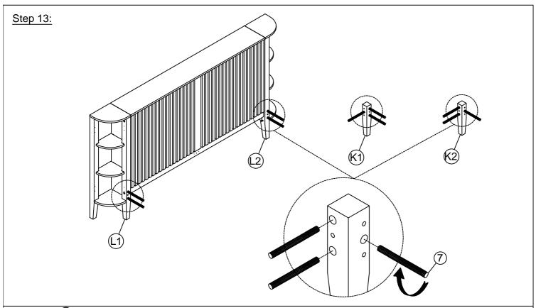
Attach Bolt 7 to the Leg-left footboard (K1), Leg-right footboard (K2) and Leg-left headboard (L1), Leg-right headboard (L2) as shown above.
