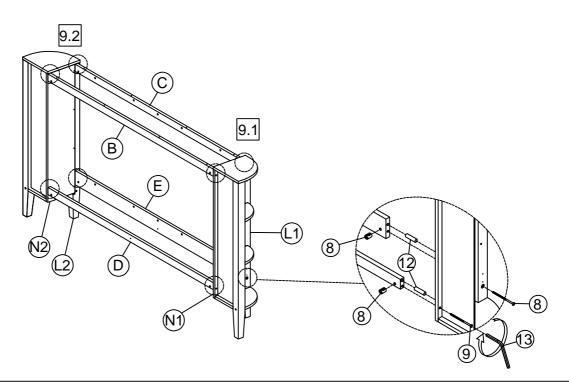
9.1: Attach Top back crossbar-headboard (B), Top front crossbar-headboard (C), Bottom back crossbar-headboard (D), Bottom front crossbar-headboard (E) to the Leg-left headboard (L1), Side left headboard panel (N1) by using Bolt(8), Bolt(9), Wooden dowel (12) with Allen Wrench (13) as shown above.
