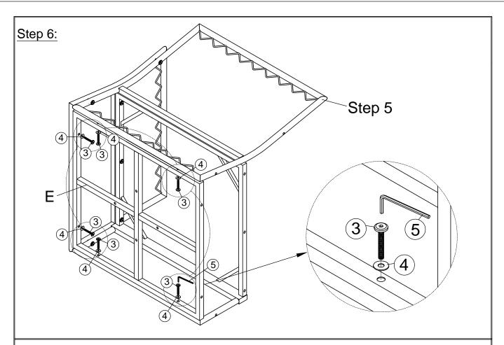
Two adults turn the frame. Fix the Rectangular frame E to the frame in Step 5 by using bolts ③, flat washers ④, and the allen wrench ⑤. **Do not fully tighten the bolts.**
