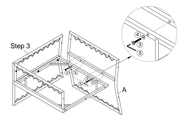
Fix the backrest panel A to the frame in Step 3 by using bolts 3, flat washers 4, and the allen wrench 5. **Do not fully tighten the bolts.**
