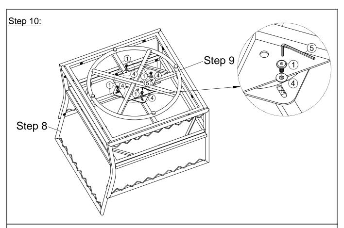
Two adults turn over the chair frame, and insert the frame in Step 9 on the chair frame in Step 8 by using the bolts 1, flat washers 4, and the allen wrench 5 to fix them. Fully tighten all the bolts in this chair frame.
