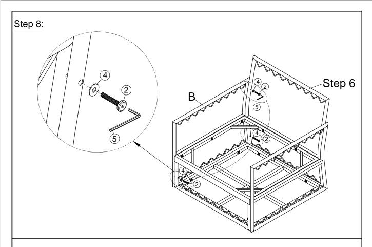
Using the bolts ②, flat washers ④, and the allen wrench ⑤ to fix the left arm panel B to the frame in Step 6. **Do not fully tighten the bolts.**
