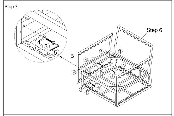
Two adults turn over the chair frame. Fix the left arm panel B to the frame in Step 6 using bolts ③, flat washers ④, and the allen wrench ⑤. **Do not fully tighten the bolts.**
