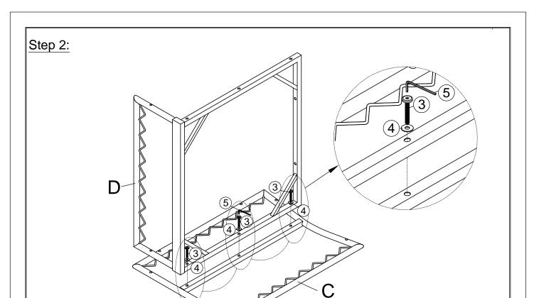
Using bolts 3, flat washers 4, and the allen wrench 5 to connect the right arm panel C to the seat panel D. **Do not fully tighten the bolts.**
