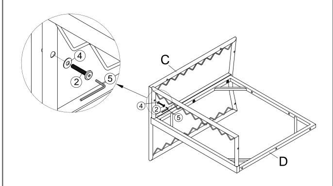
Using bolts ②,flat washers ④, and the allen wrench ⑤ to fix the right arm panel C to the seat panel D. **Do not fully tighten the bolts.**
