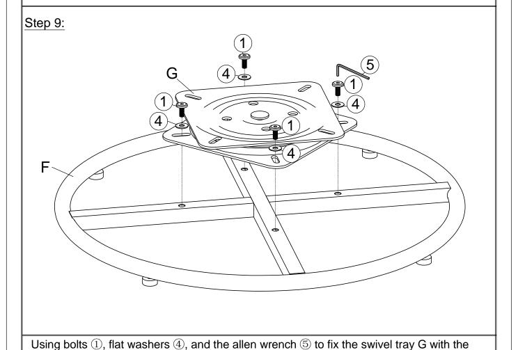
round frame F. Fully tighten the bolts.
