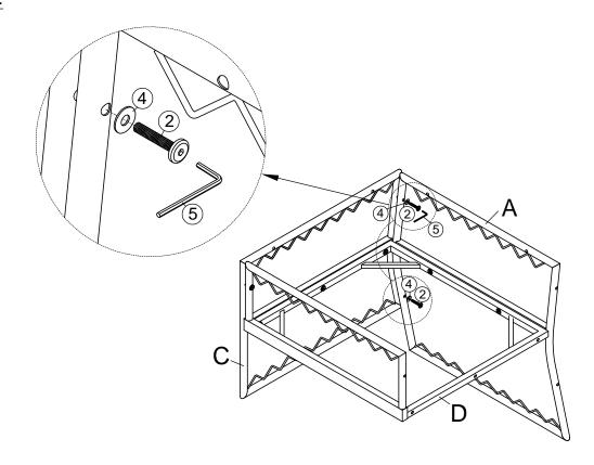
At the intersections of the backrest panel A and the right arm panel C, using bolts ②, flat washers ④, and the allen wrench ⑤ to fix the frame. **Do not fully tighten the bolts.**
