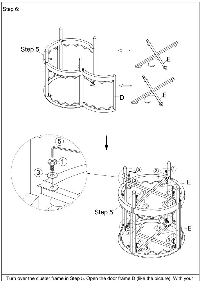
adult partner, put the support frame E under the pats in this direction. Using bolts ①, flat washers ③, and the allen wrench ⑤ to fix Support frame E to the table frame.
