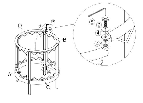
Using bolts ②, plastic flat washers ④, and the allen wrench ⑤ to fix the door frame D with the cluster frame in Step 3. **Fully tighten all the bolts in the table frame.**
