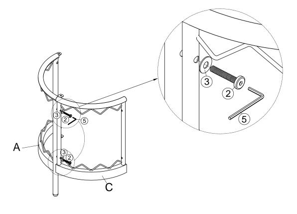
Using bolts 2, flat washers 3, and the allen wrench 5 to fix 2 frames A and C. **Do not fully tighten the bolts.**
