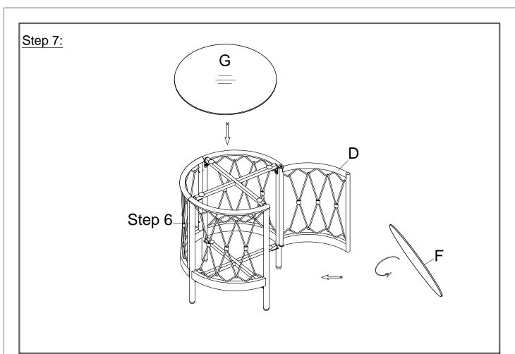
Open the door frame D. Turn the bottom glass F and put it on the bottom support braces. The top glass G is put on the top support braces.
