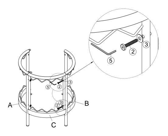
Fix the frame in Step 2 with the leg frame B using bolts ②, flat washers ③, and the allen wrench ⑤. Do not fully tighten the bolts.
