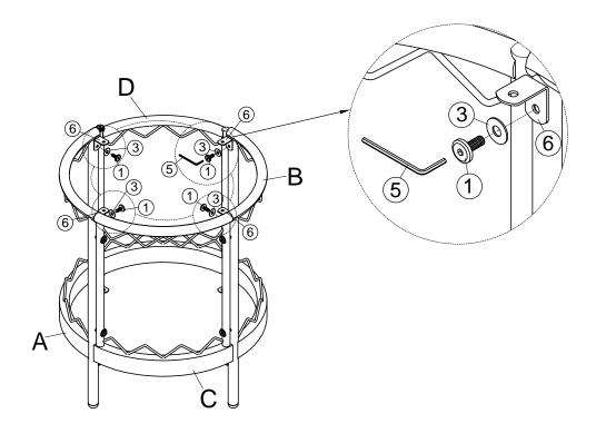
Connect pats 6 at frame A and B's legs by using bolts 1, flat washers 3, and the allen wrench 5. Fully tighten the bolts.
