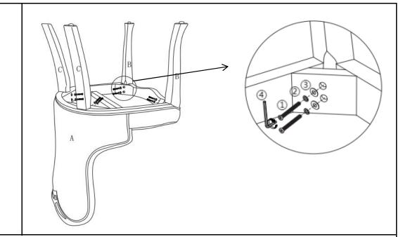
Place the Seat with Back (A) on the side of a table with the Seat facing down, as seen in the picture.
