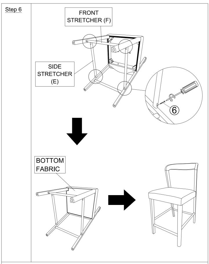
Secure Side Strecher (E) and Front Stretcher (F) using Csk Screw (6). Re-cover the fabric under the seat. Your counter stool is ready to use.
