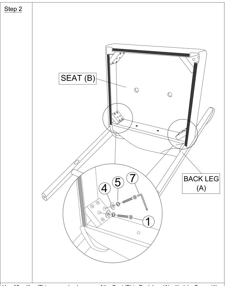
Use Allen Key (7) to secure back corner of the Seat (B) to Back Leg (A) with Jcbc Screw (1), Spring Washer (5) and Flat Washer (4).
