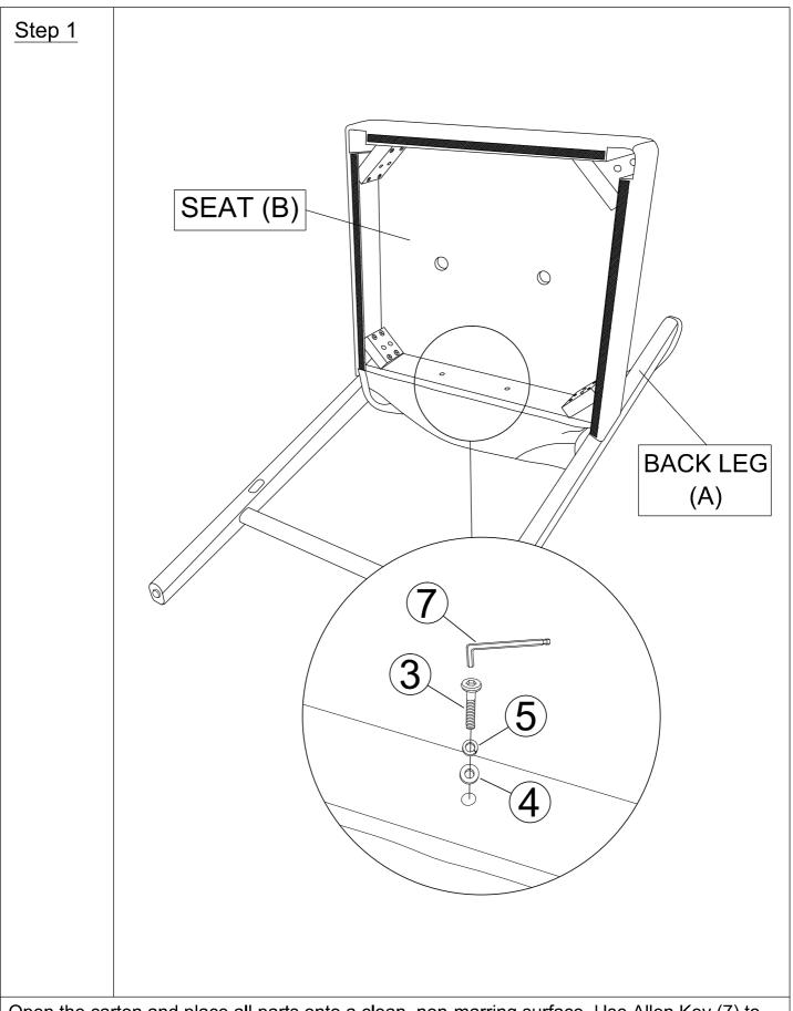
Open the carton and place all parts onto a clean, non-marring surface. Use Allen Key (7) to secure Seat (B) to Back Leg (A) with Jcbc Screw (3), Spring Washer (5) and Flat washer (4).
