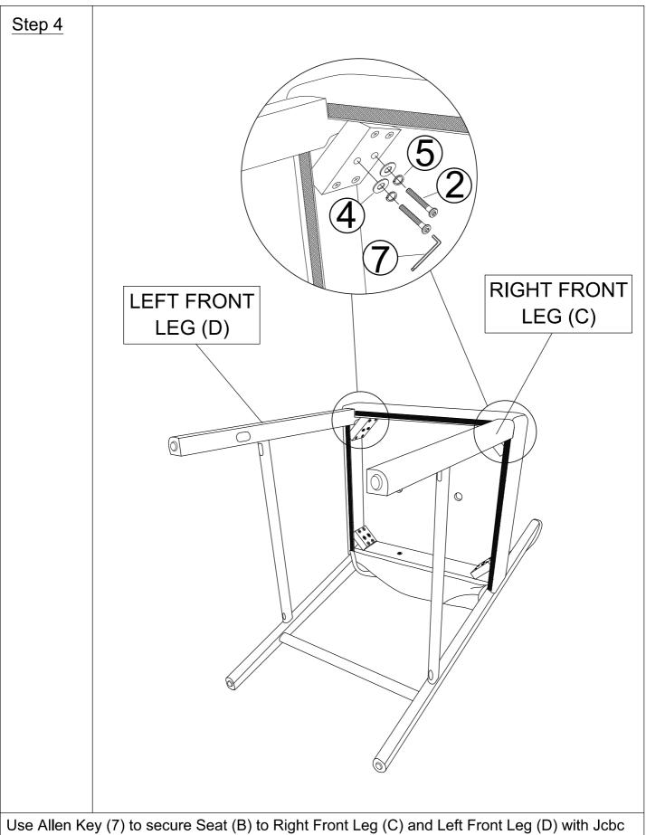
Use Allen Key (7) to secure Seat (B) to Right Front Leg (C) and Left Front Leg (D) with Jcbc Screw (2), Spring Washer (5) and Flat Washer (4).
