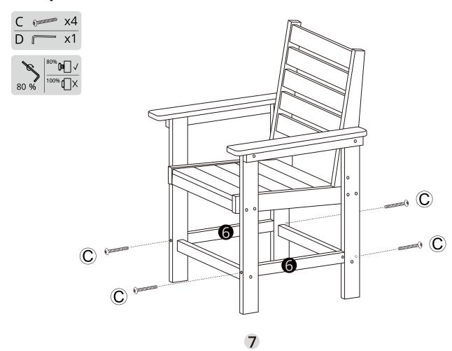
Now you can 100% tighten all bolts in Step 1 2 3 4 5 6 to ensure a steady use of the item.
