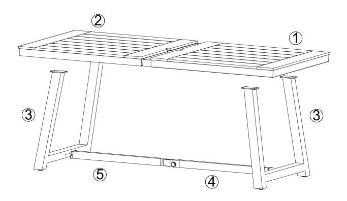
1 Insert table frame ① into table frame ②, then lock the two table frames.
