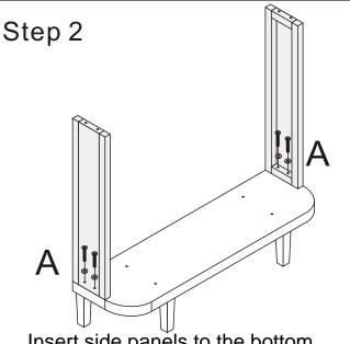
Insert side panels to the bottom.
