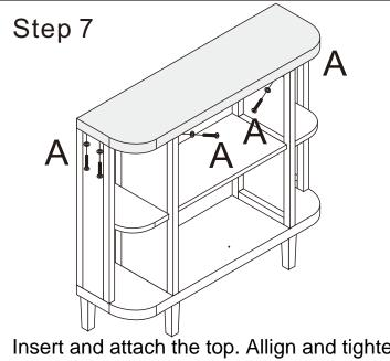
Insert and attach the top. Allign and tighten screws & washers by Allen Wrench
