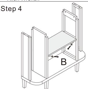
Insert the mid shelf board to the mid panels. Allign and tighten screws & washers by Allen Wrench
