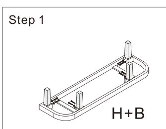
Insert and screw in the cabinet feet to the bottom board
