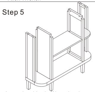
Insert the side shelf board to the panels. Allign and tighten screws & washers by Allen Wrench
