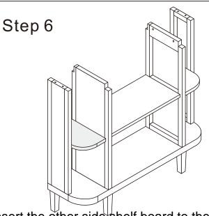
Insert the other side shelf board to the panels. Allign and tighten screws & washers by Allen Wrench
