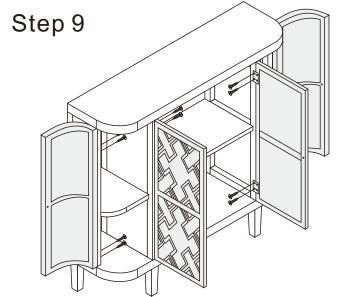
Install the doors by screw in to the panel with screw driver.
