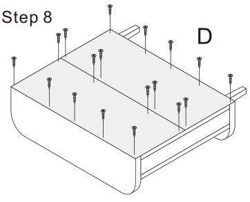
Align back panel and screw in by screw driver.
